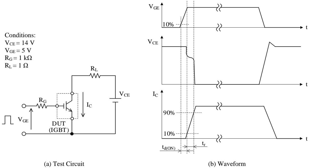
Figure 3. Switching Time Test in Resistive Load
