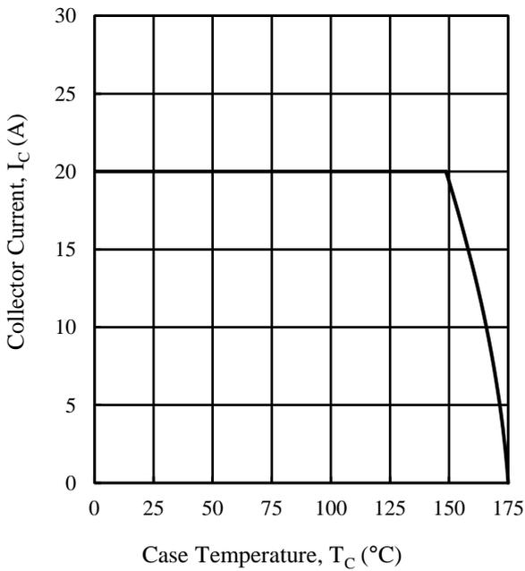
Figure 7. Typical Characteristics:  $I_C$  vs.  $T_C$  ( $V_{GE} = 5$  V)
