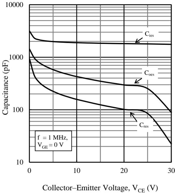
Figure 17. Typical Characteristics:
