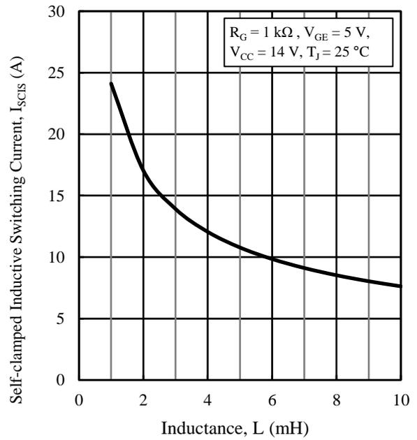
Figure 16. Typical Characteristics:  $I_{SCIS}$  vs.  $L$
