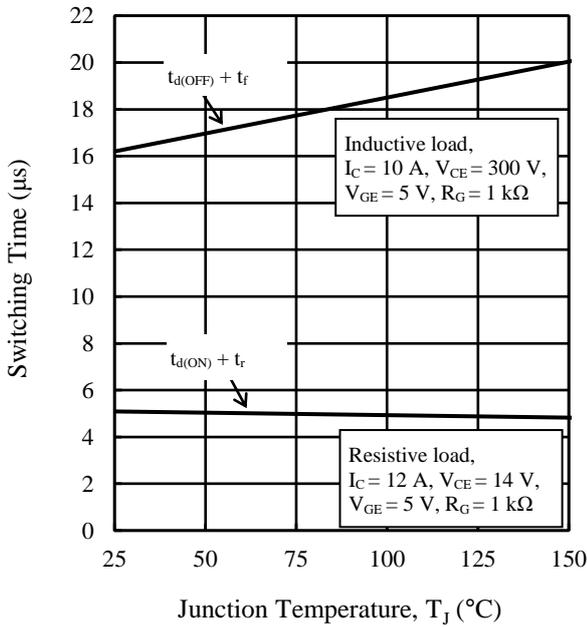
Figure 19. Typical Characteristics:
