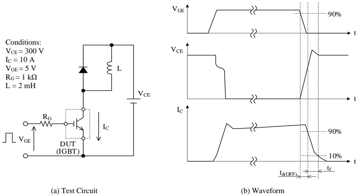
Figure 4. Switching Time Test in Inductive Load
