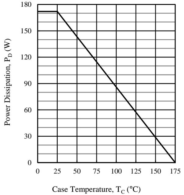
Figure 6. Typical Characteristics:  $P_D$  vs.  $T_C$
