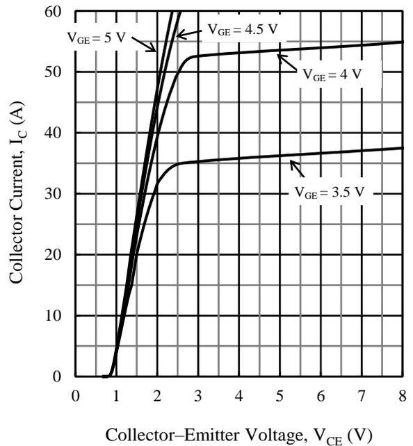
Figure 8. Typical Characteristics:  $I_C$  vs.  $V_{CE}$  ( $T_J = -40$  °C)
