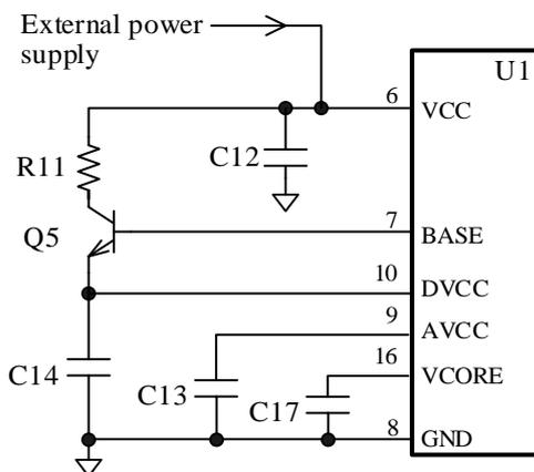
Figure 8-2. Power Stage and Its Peripheral Circuit
