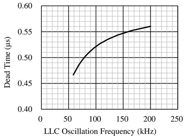
Figure 8-19. Dead Time vs. LLC Oscillation Frequency
