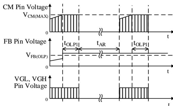
Figure 8-20. Operational Waveforms of LCC\_OCP and LCC\_OLP
