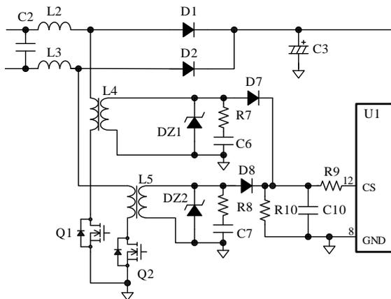
Figure 8-4. CS Pin and Its Peripheral Circuit
