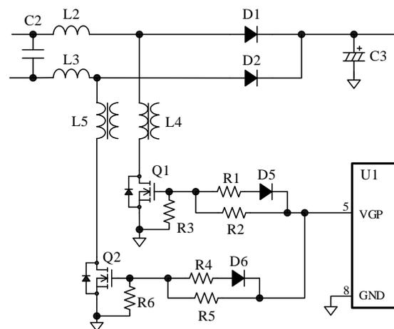
Figure 8-1. VGP Pin and Its Peripheral Circuit
