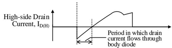
Figure 8-18. Point to Be Checked in ZCS
