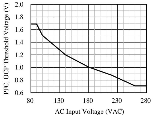
Figure 8-12. PFC\_OCP Threshold Voltage vs. AC Input Voltage
