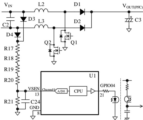
Figure 8-10. VSEN Pin and Its Peripheral Circuit
